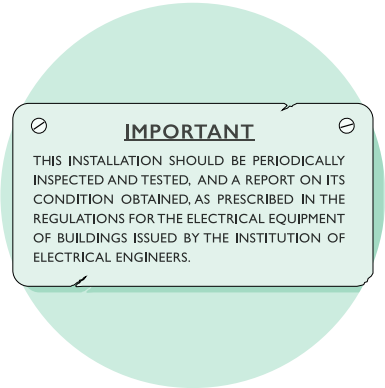
A typical periodic inspection notice for an older installation
